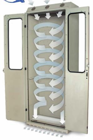
The unique design of the SureDry Scope Cabinet includes both top fans for intake and lower fans for exhaust. This push/pull design creates a vortex of air that flows through the cabinet ensuring maximum drying efficiency.
