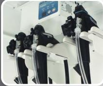
All SureDry scope cabinets are fully designed to be purchased with Dri-Scope Aid®, the industry best lumen drying system, or field installed with easy "Plug & Play" installation to provide HEPA filtered air to each internal scope channel.
