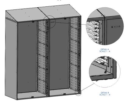
and bottom. With one cabinet already mounted to the wall, move your second cabinet into place directly adjacent to it. Once in place, make sure that the pre-drilled side holes within the first cabinet line-up perfectly with the pre-drilled holes of the second cabinet.
