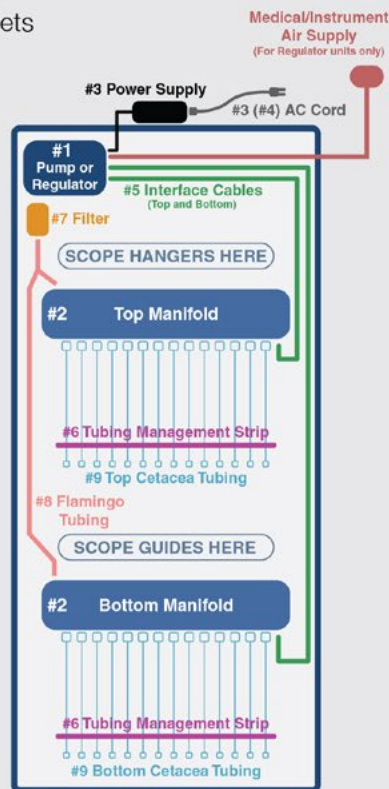
Finished upgrade for a 10 scope cabinet
